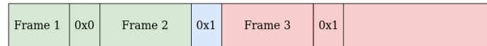
(b) Persistent stack after writing the new frame after the stack end marker
